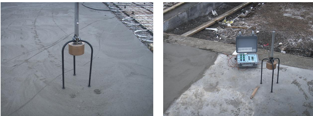
Figure 7. Penetration test device (left) and temperature logger (right).
